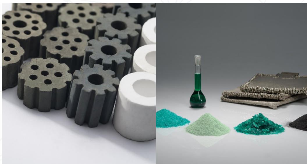
▲ Different Types of Nickel Based Natural Gas Reforming Catalysts (left) and All Pure Derivatives of Recovered Nickel from Spent Catalyst used in the Catalyst Manufacturing Process (Right)
